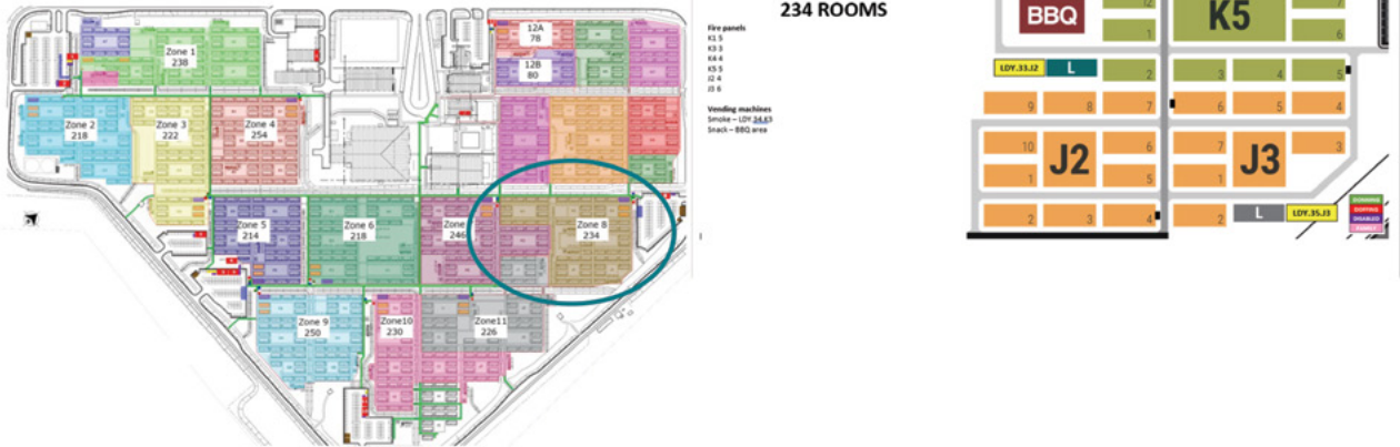
Section 3: Figure 10: Example of zone allocation for a Pod Team at Centre For National Resilience. Zone 8, contains 234 rooms with one point of entry exit for donning and doffing.
